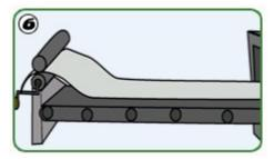
The ingots are sent to mills where they are rolled out, this gives the aluminium greater flexibility and strength.
